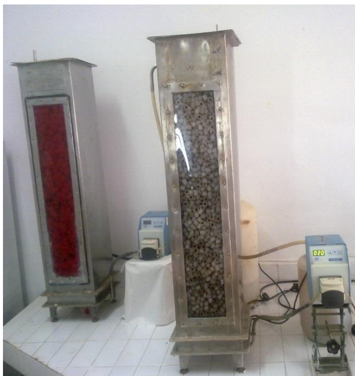
Figure 3. Experimental anaerobic bioreactor system.
